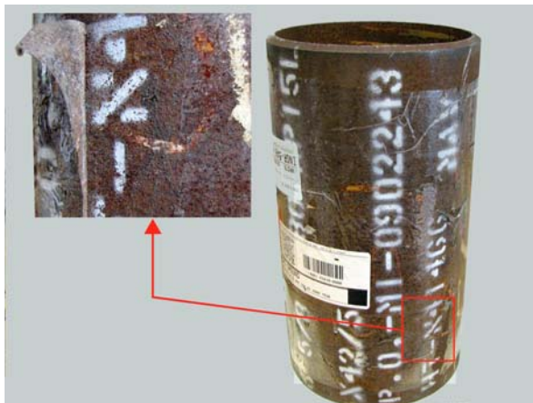
Figure 10 - Section of 6 in. diameter API 5L piping used for evaluating corrosion removal performance of bristle blasting tool
